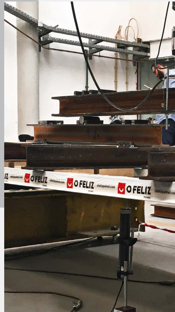
Full panel bending test
